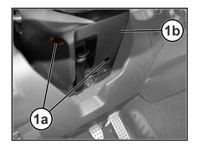
3. Remove the steering column lower shroud (1a) by releasing the internal retainers (1b).
